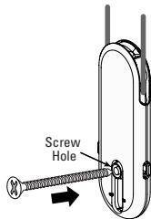
c. Press in on the UCT release buttons and pull down on the screw hole to align the hole with the wall anchor or pilot hole.
