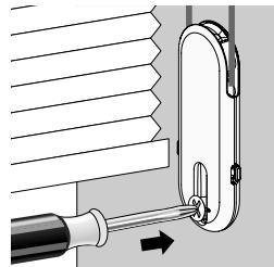
**CAUTION:** Do not overtighten the mounting screw. This can prevent the UCT from functioning properly and increase cord wear.
