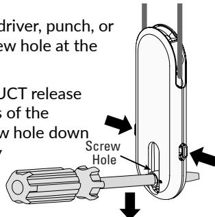
3. Slide the UCT down to the bottom of the cord loop.
