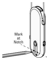
4. Hold the IB bracket with its center hole aligned with the mark and mark both hole locations.
