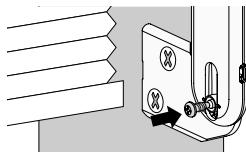
8. Ensure the cord can move freely through the UCT without engaging the lock. The center of the screw hole should be aligned with the notch in the UCT ( $\pm 1/8"$ ).
