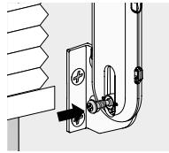
8. Ensure the cord can move freely through the UCT without engaging the lock. The center of the screw hole should be aligned with the notch in the UCT ( $\pm 1/8"$ ).
